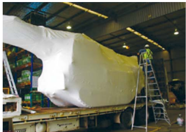
Drill rig wrapped after cleaning, to maintain quarantine compliance during transport to Barrow Island
